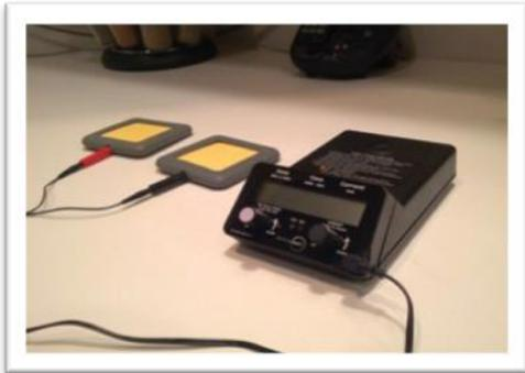
Fig. 3 - Portable stimulator DC, equipped with a pair of electrodes (supplier Scriphessco)
